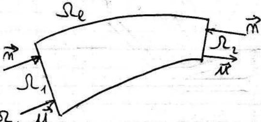
$$M = \int_S \rho \vec{u} \cdot \vec{n}_m dS = P \int_{S_1} \vec{u} \cdot \vec{n}_m dS + P \int_{S_2} \vec{u} \cdot \vec{n}_m dS + P \int_{S_L} \vec{u} \cdot \vec{n}_m dS$$
