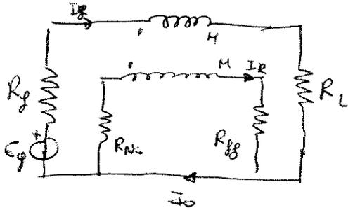
$$\begin{cases} E_g = I_g(R_g + R_L) + j\omega M I_r \\ j\omega M I_g = (R_{ng} + R_{fg}) I_r \end{cases}$$
