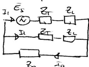
$$\begin{cases} \bar{E}_s = (Z_T + Z_L) I_1 + Z_0 (I_1 + I_2) \\ 0 = (Z_T + Z_L) I_2 + Z_0 (I_1 + I_2) \end{cases}$$
